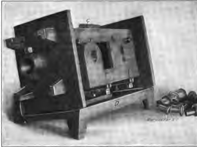
Fig. 25. Jig in Fig. 24 in Position for Drilling Holes at an Oblique Angle with Jig Base
